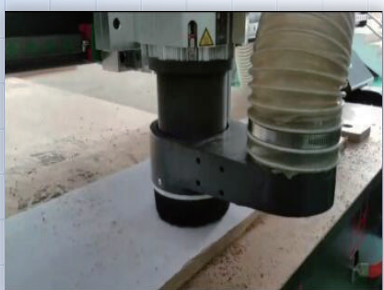
Dust Tracker Dust hood will go up and down according to the cutting depth, to provide the cleanest cutting.
