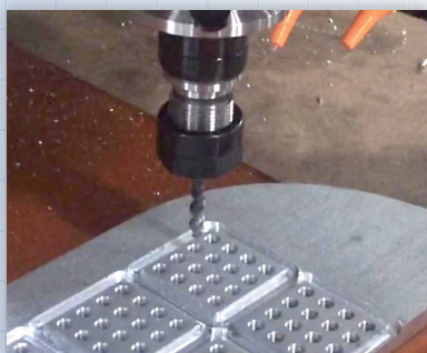
Drilling and Tapping By spindle
